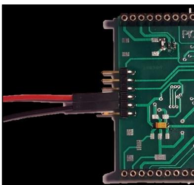
The PICado Alpha 2 Development Board can be powered with an external 5V power supply connected to the programmer pins.
