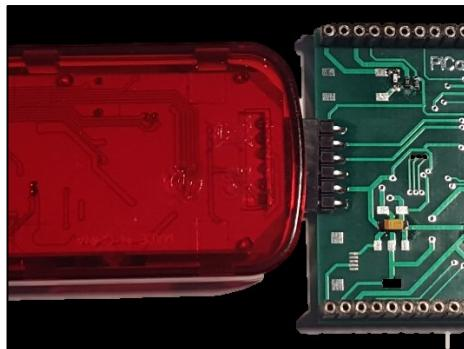
Microchip's PICkit 3 In-Circuit Debugger/Programmer uses in-circuit debugging logic incorporated into each chip with Flash memory to provide a low-cost hardware debugger and programmer.
