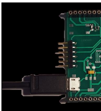
The PICado Alpha 2 Development Board can be powered with an external 5V micro USB power supply.
