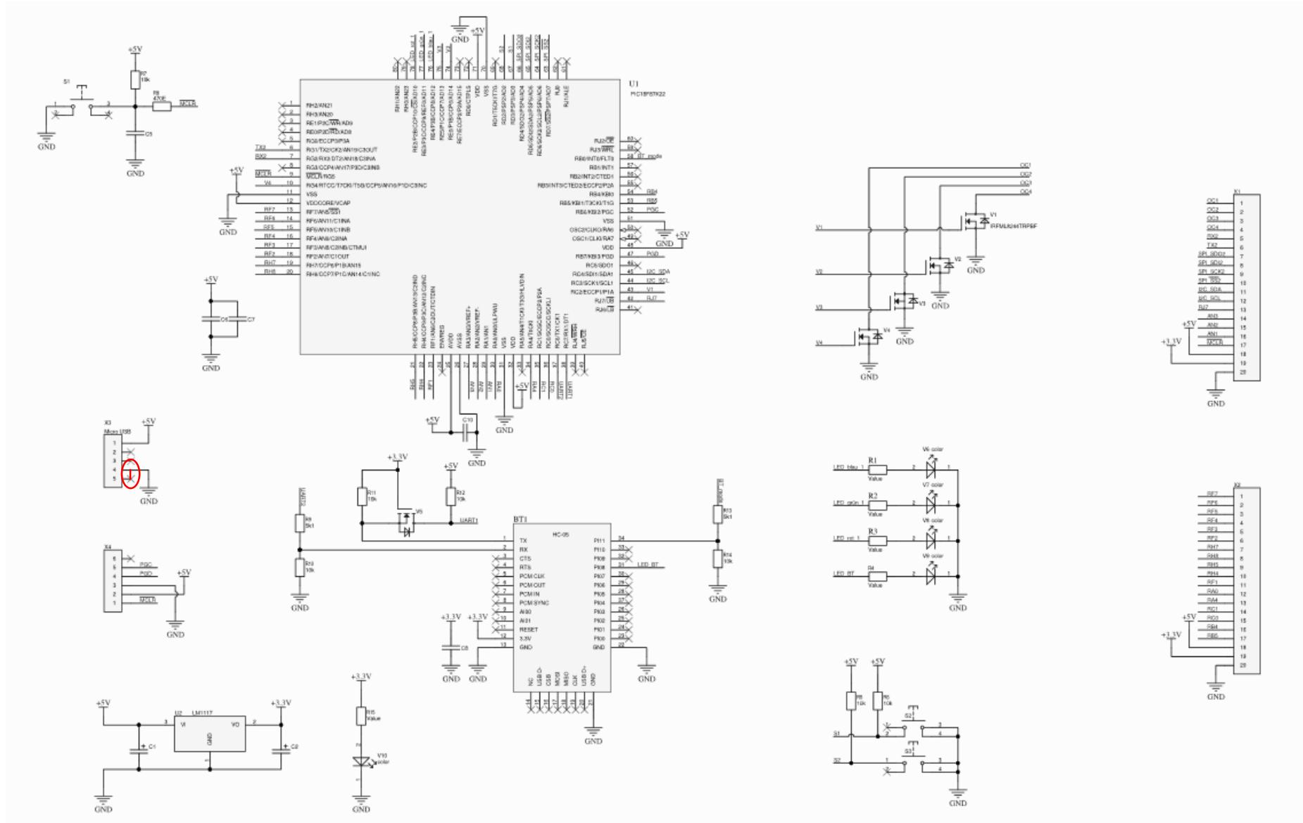
To use the PICado Alpha 2 as a 5V board you must short X6 and the tow pins of the X2.
