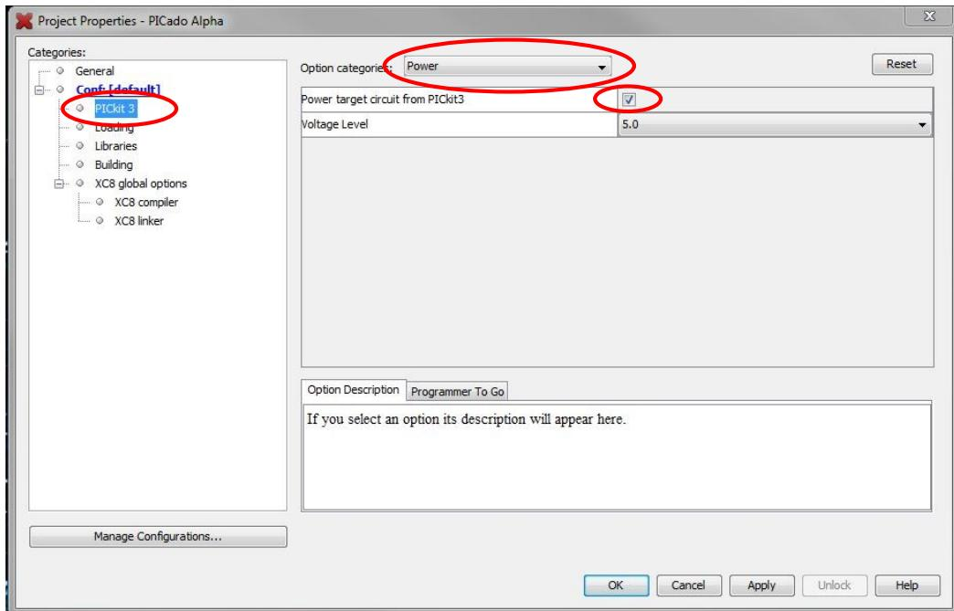
The PICado Alpha 2 Development Board can also be powered with a PICkit or ICD programming device.
